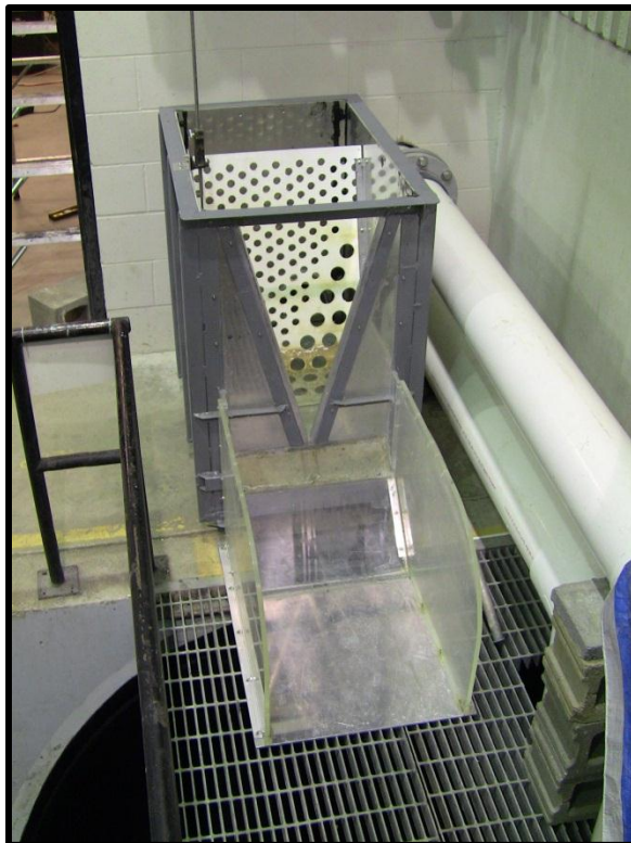
Figure 3-8 V-Notch weir tank
